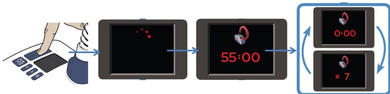
Connect the machine to the mains once tubing is in place. Press the button and the disinfection cycle will begin. This will take 55 mins, when it has finished the count will be at 0:00. At this point turn the machine off BEFORE turning the power off at the wall.
