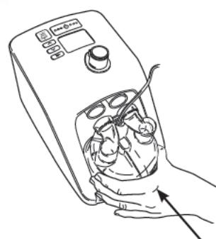
d).Depress the front lip of the machine and slide the chamber inside, ensuring that the adaptor connects onto machine correctly, as above.
