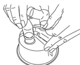
b).Pull the drip line over the front of chamber along the central groove. Then connect the clear adaptor as above.
